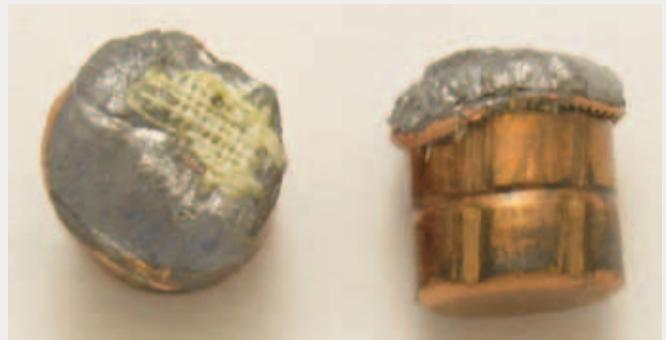
9mm FlexLock bullet fired through glass
