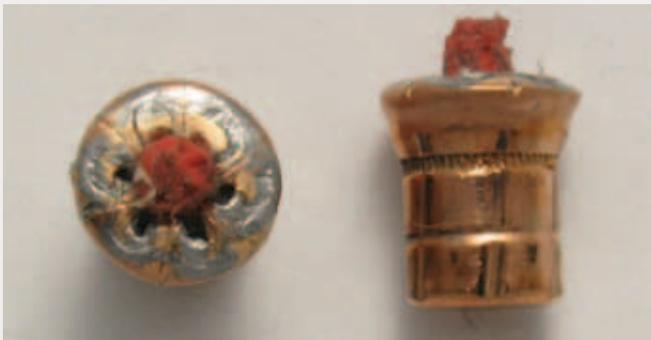
9mm FlexLock bullet fired through sheet metal
